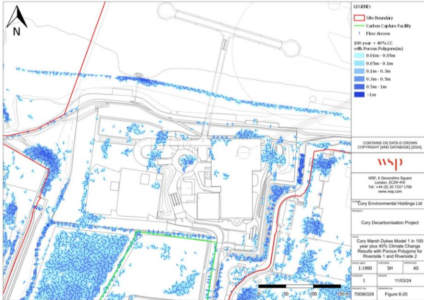
Figure 8-20: Cory Marsh Dykes Model 1 in 100 year plus 40% Climate Change Results with Porous Polygons for Riverside 1 and Riverside 2
